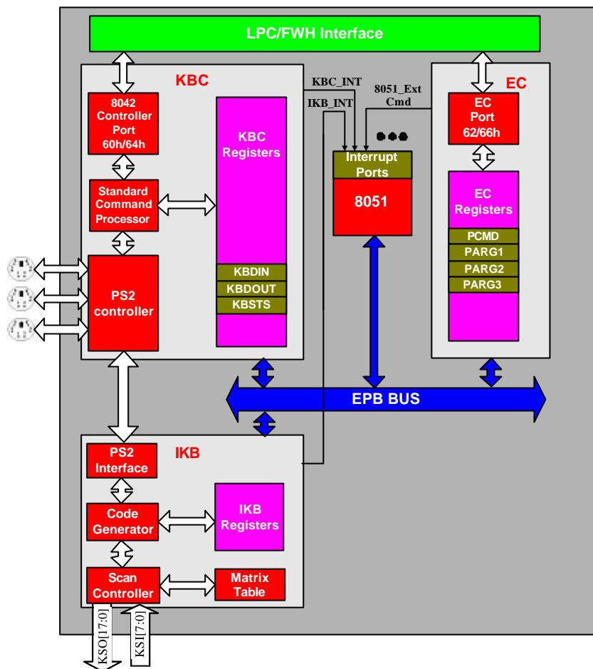
Standard KBC or EC commands will be automatically processed by hardware with result stored into **KBCOUT** and status updated in **KBCSTS**. Extended KBC commands will be forwarded to 8051 (by generating interrupt) for processing via registers **KBCIN**, **KBCOUT** and **KBCSTS**.
