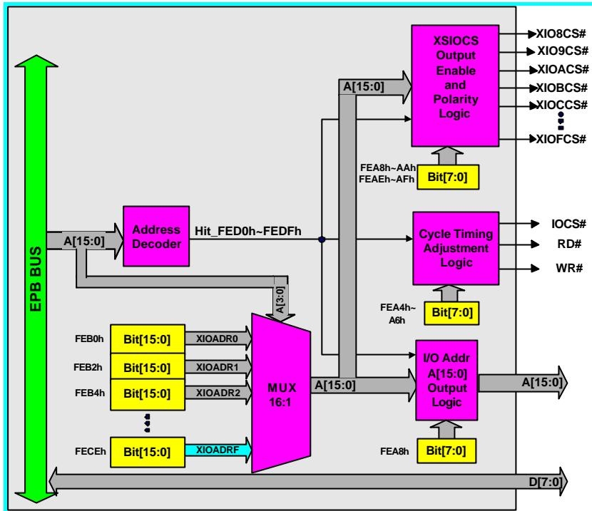
The XIO module interfaces to external IO devices via the XBI interface with programmable addresses defined in registers **XIO\_A8~F**(FEC0h~CFh). For example, assuming **XIO\_A8** contains “1060h”, when there is a write cycle toward the XIO8 port(FED8h), an IO write cycle will be taking place on XBI bus with **A[15:0]**=“1060h”, and the host data appearing on **D[7:0]**.
