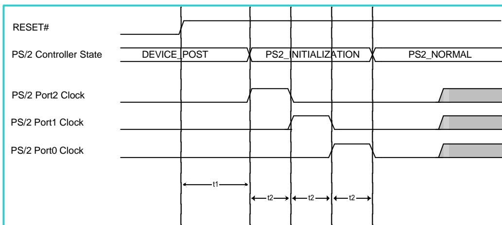
(Power-On Self Test) by themselves. After DEVICE-POST state, KB3910 will go to PS/2-INITIALIZATION state, during which state the KB3910 will detect and initialize PS/2 devices that are already plugged-in. Finally, KB3910 will go to PS/2-NORMAL state, during which state KB3910 will be in operational state. The waveforms are demonstrated as follows.
