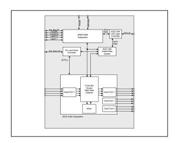
**DICE Mini** is a monolithic CMOS ASIC capable of receiving and transmitting up to 16 channels of audio data in accordance with the **IEEE 1394** standard.
