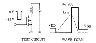
$$\begin{array}{l} T_{ch} = 25^{\circ}C \text{ (Initial)} \\ \text{Peak I}_{AR} = -11 \text{ A, } R_G = 25 \text{ }\Omega \end{array} \quad \text{EAS} = \frac{1}{2} \cdot \text{L} \cdot \text{I}^2 \cdot (\frac{\text{BVDSS}}{\text{BVDSS} - \text{VDD}}) \\ \text{VDD} = -24 \text{ V, L} = 1.0 \text{ mH} \end{array}$$
